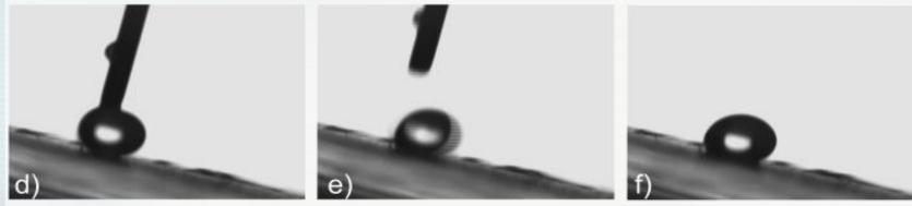
Adhesive force of oil in water. a-c) A droplet of diiodomethane rolling off the micro/nano-structured ZnO surface as soon as the droplet made contact. d-f) Onto the fluorinated surface the drop firmly adhered to the surface and did not roll away indicating a Wenzel state. Roll off angle was ~10°.
